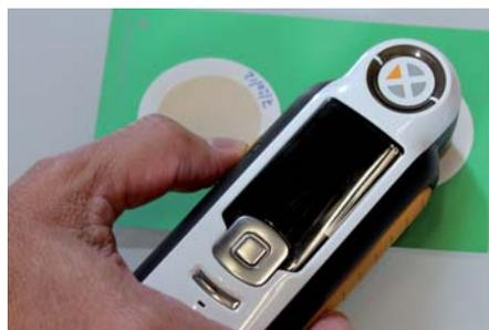
MPC-Test (Membrane Patch Colorimetry)
